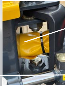
Protected hose lines
