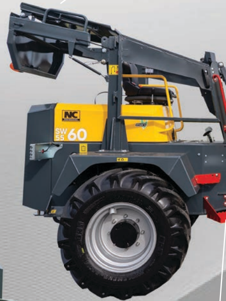
Highlighted Steps + Handrails
