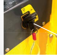
Two stage start inhibitor safety system
